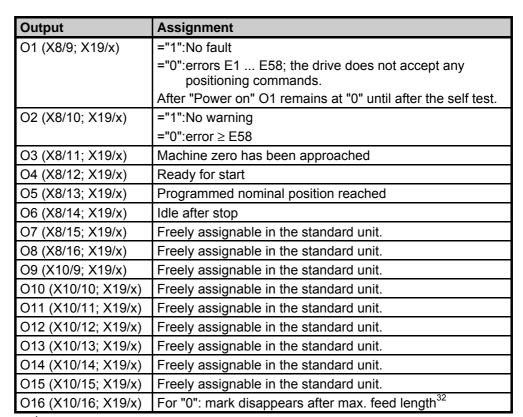
The assignment of outputs on X19 applies only to COMPAX 1000SL.
